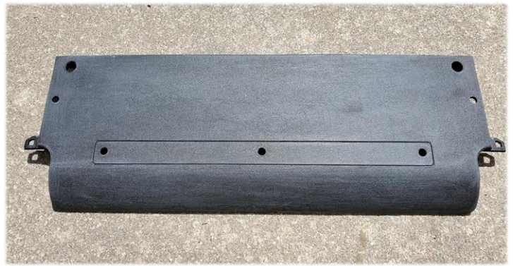
The cleaned and stripped plastic front seat panel
